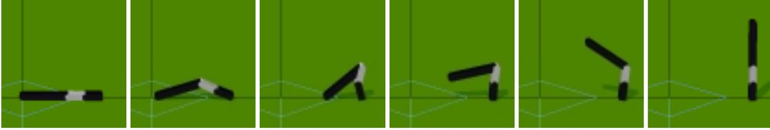
Figure 5. Example of a successful stand-up trajectory
