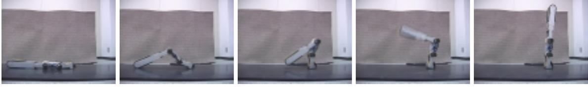
Figure 11. Example of a stand-up trajectory using the real robot
