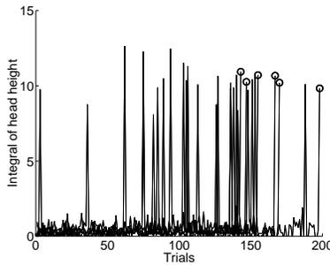
Figure 9. Time course of learning with the real robot. Circles show 10th successful stand-up in which a simulation run was terminated.
