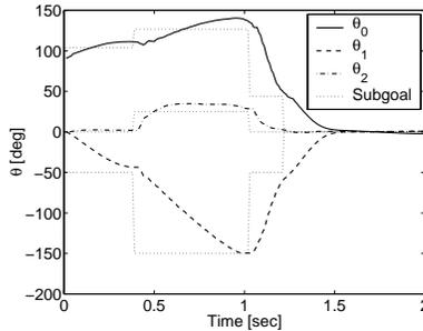
Figure 10. Example of a time course of a stand-up trajectory and a sub-goal sequence ( $\theta_0$ :pitch angle,  $\theta_1$ ,  $\theta_2$ :joint angle)
