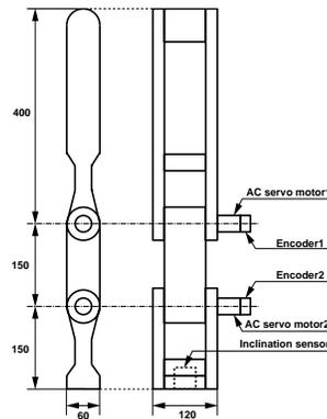
Figure 8. Real robot configuration
