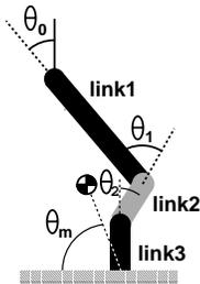
Figure 1. Robot configuration.  $\theta_0$ :pitch angle,  $\theta_1$ :hip joint angle,  $\theta_2$ :knee joint angle,  $\theta_m$ :the angle of the line from the center of mass to the center of the foot.
