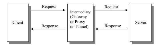
Figure 1. Use of intermediary in HTTP communication Model
