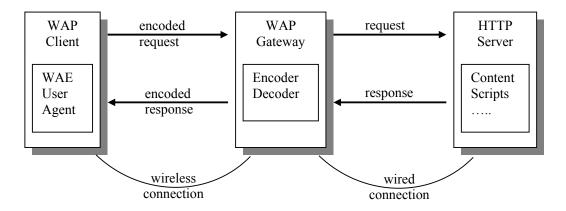
Figure 3. WAP infrastructure using intermediate gateway
