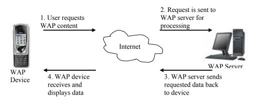
Figure 2. Direct communication between WAP Device and WAP Server
