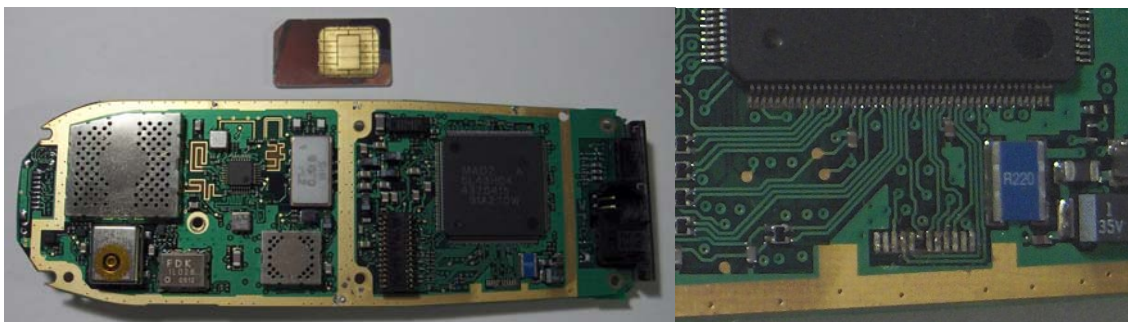
Figure 9: 5110 system board with JTAG test points.
