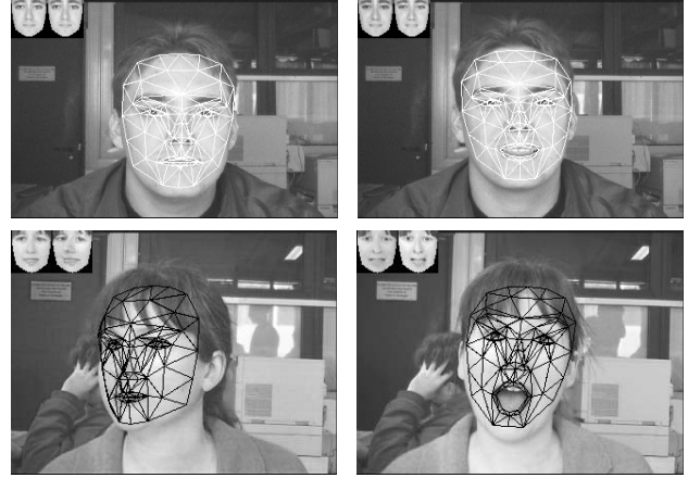
Figure 4. Face and facial feature tracking results associated with two sequences. The second sequence features illumination variations.
