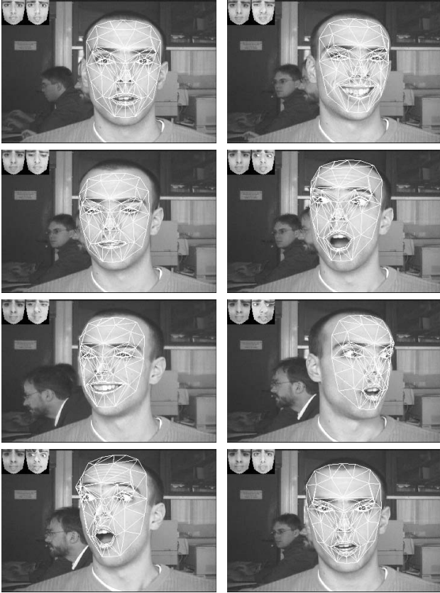
Figure 2. Face and facial tracking results. Frames 63, 181, 222, 282, 418, 492, 522, and 683, 720x480 pixels in size, in a 750-frame-long sequence. The upper left corner shows the current appearance A_t and the shape-free texture.
