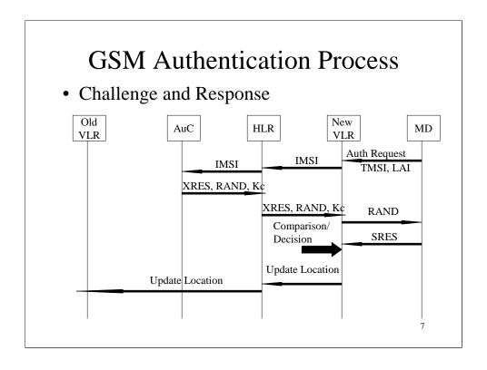
When the mobile phone is switched on, a challenge and response session is started to control the validity of the data. The MS transmit the registration request to the base station and the BTS forwards the request to the MSC which informs the Corresponding VLR on the user's location. The request includes the Temporary mobile subscriber id and the LAI.
