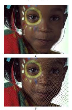
Fig. 3. Image decoded with errors due to unreliable data transmission line: a) for the standard JPEG, PSNR=24.05 dB, b) for the standard JPEG2000, PSNR=23.98 dB
