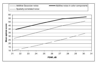
Fig. 6. Dependences of the MOS on PSNR for different spatial frequency and color distributions of additive noise
