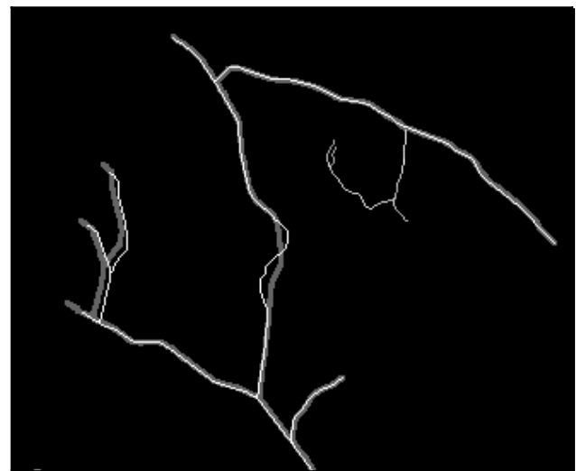
fig. 9. Change detection image. Solid white lines represents the old road database. Grey ribbons the new delineation of the old roads. New road pixels are represented by grey levels corresponding to their level of significance.
