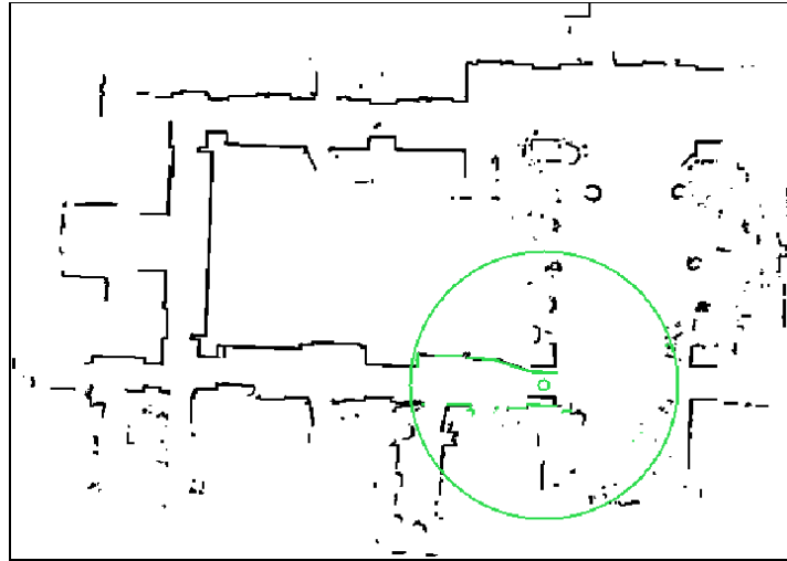
Figure 13. A partial map of a wing of the Computer Science Building at Stanford University. The total length of the circuit is approximately 40 meters. The circled region corresponds to the last local measurement.
