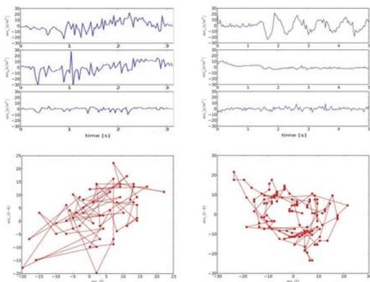
**Figure 5.** Left column incorrect bowing, right column correct bowing, time series of accelerations along the x-, y-, z-axis and below Takens embedding, plotting accelerations against their delayed values.
