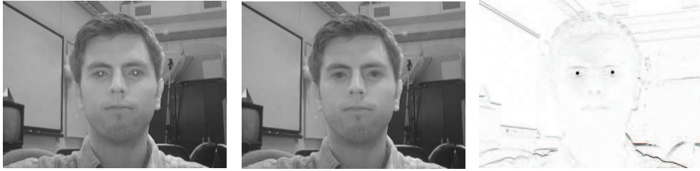
Figure 2. Left: the bright image, Center: the dark image, Right: Difference Image (contrast enhanced)
